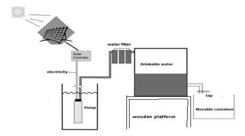
The given process illustrates how underground water is pumped out and made fit for drinking by using energy from the sun. It can be seen that mainly four steps are involved in the process.
