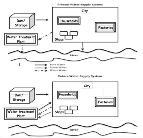
The given pictures illustrate Australia's current water supply system and the changes proposed to it in future. It can be seen that the changes proposed are for better recycling of water, and also the wastewater will not be released into the river.
