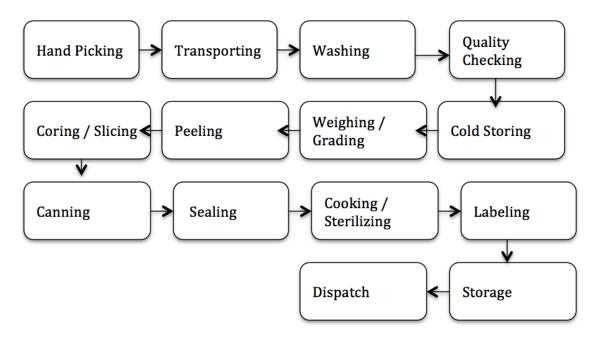
The diagram illustrates how to produce canned fruit step by step. It is clear that there are several main steps in the process, from the picking of the pears to the final canned product.
