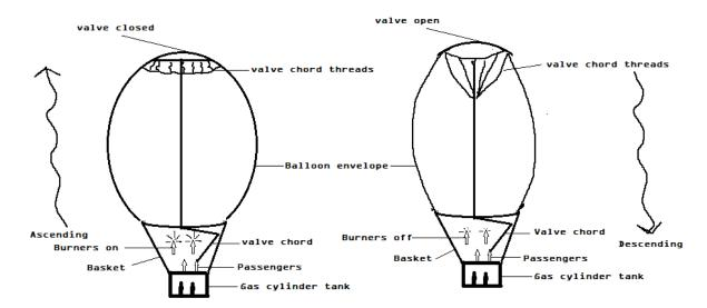
The given picture illustrates the working of a hot air balloon. It is evident that to make the balloon descend, the burners have to be extinguished.
