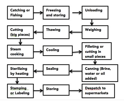
The given picture illustrates the process of canning of fish. It is manifest from the graph that 15 steps are involved from the initial catching to the final dispatch to supermarkets.
