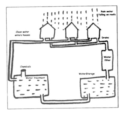
The given diagram illustrates how rainwater is harvested to use as drinking water in an Australian town. A quick glance at the diagram makes it clear that rainwater is filtered and also treated chemically before sending it back to the houses for use by the people.
