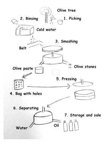
The given process depicts the stages in the production of olive oil. It is clear from the picture that there are seven main stages from the picking to the final sale.
