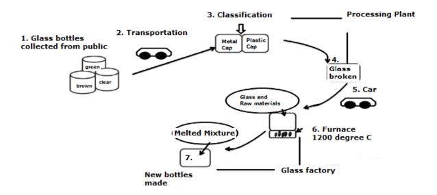
The given picture illustrates the stages in the recycling of glass bottles. It is clear that seven steps are involved in the process.
